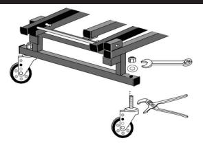
Attach swivel casters as shown. While tightening lock nuts, grip bearing cap with channel lock pliers or pipe wrench to prevent threaded stem from turning. Tighten lock nuts firmly, but not excessively tight. Check lock nut tightness on caster stems periodically.
