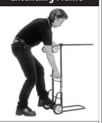
Loosen wingbolts 1/4 turn. Step on rear axle and push in extension stop button. Pull up on frame as shown until stop button engages. Retighten wingbolts.
