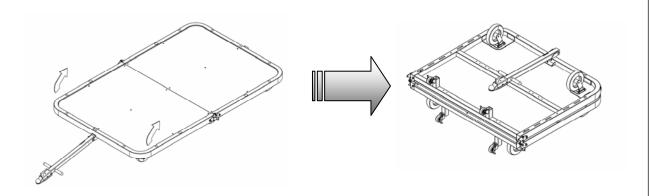
Rotate the hitch tube so that it rests on the floor. Pick up on the front half of the cart and rotate it onto the back half. Position the hitch tube as shown and reinsert threaded studs for storage. **Note: Cart can be** maneuvered manually with hitch tube in this orientation. Be sure to have plenty of room when folding cart.
