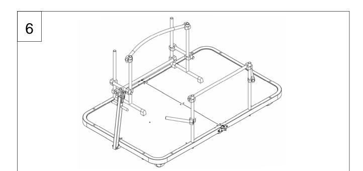
With the vertical rails attached tube clamps can be used to position the remaining horizontal equipment rails. The orientation of these rails can be altered for a wide variety of performance setups.
