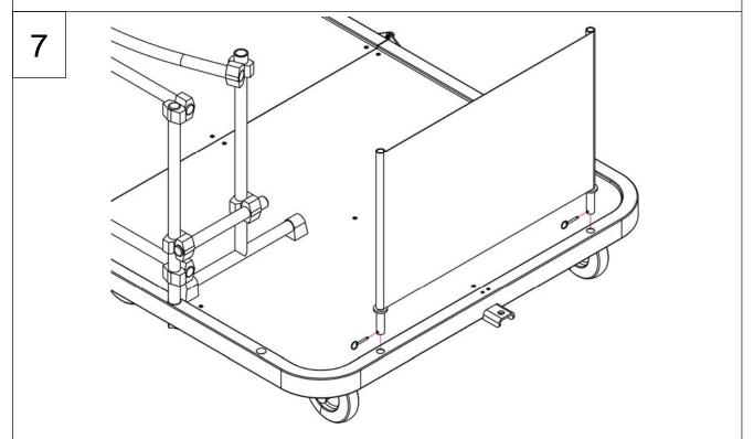
To attach vinyl surrounds insert vertical posts through the proper hole in the top of the frame tube. Use the supplied pins and pin through the hole in the vertical posts, on the underside of the Field Cart.
