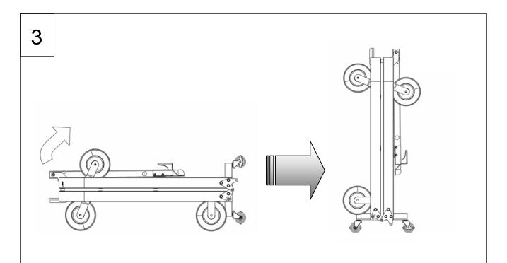
Lift up on the front end of the cart to rotate onto the storage casters. Now the cart can be pushed or pulled to the desired storage location. *Note: Remove threaded studs before unfolding cart when going from the storage position to the use position.*
