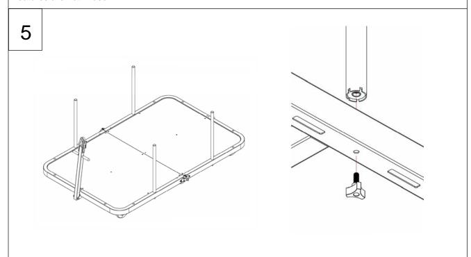
To add equipment rails insert the vertical rail tubes through the top of the frame tube. Use the supplied hardware to securely fasten the rail tube to the frame.
