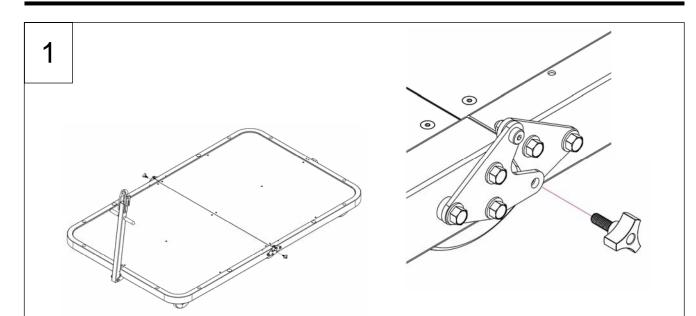
To fold the Field Cart up for storage, begin by removing the locking stud from both sides of the cart. Turning the plastic knob counterclockwise will remove the stud while turning clockwise will tighten the stud. Place the studs aside as they need to be reinserted after the cart has been folded for storage. **Note: Casters** should be in locked position when folding/unfolding the Field Cart. The process of folding/unfolding requires two people.
