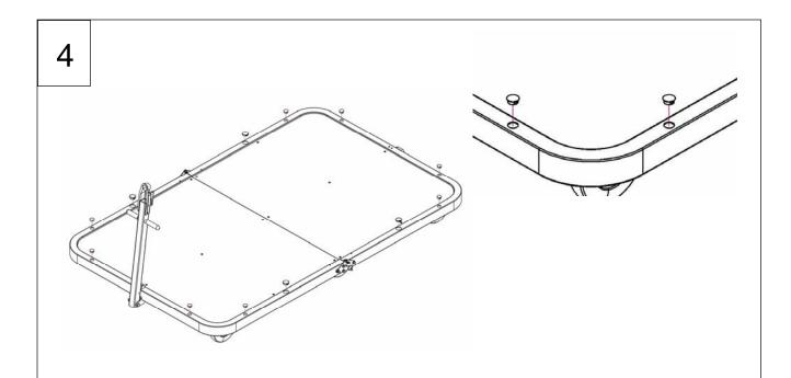
**Note:** The following steps show installation of add-on features which are sold separately. Remove plastic caps from the top of the frame tube. Plastic caps are reusable and can be reinserted when add-on features are not in use.
