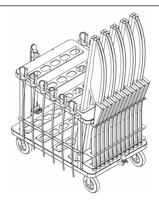
The Flag Cart equipped with the add-on features is capable of hauling 80 marching band flags, 12 sabers and 12 rifles. Use the supplied bungee cord to secure rifles before moving cart.
