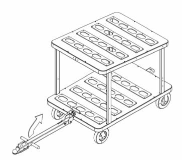
Raising the hitch tube back up will cause it to automatically lock in the upright position for storage.
