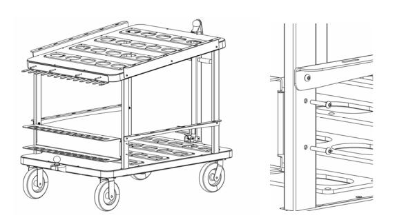
To attach optional Rifle Brackets use the supplied bolts, nuts and washers to bolt thru the frame. Four bolts are used to attach both the top and bottom rifle brackets.
