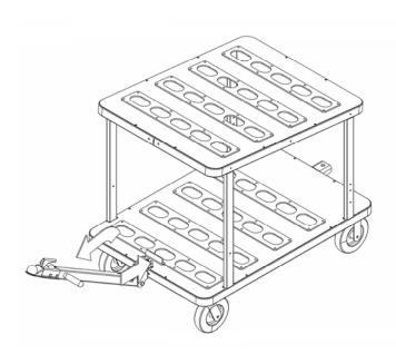
To unlock the hitch from the upright/locked position, disengage the locking mechanism by depressing the hitch latch. This allows the hitch tube to lower to its hauling position so it can be moved manually or with a hitched vehicle. Hitch has handles for manual pulling.
