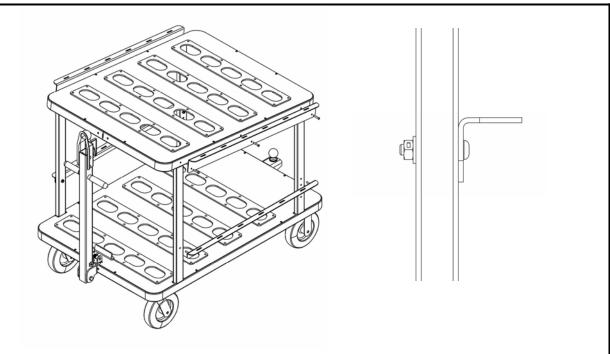
To attach optional Saber Brackets use the supplied bolts, nuts and washers to bolt thru the frame. Three bolts are used to attach the top brackets while two bolts are used to attach the bottom brackets.
